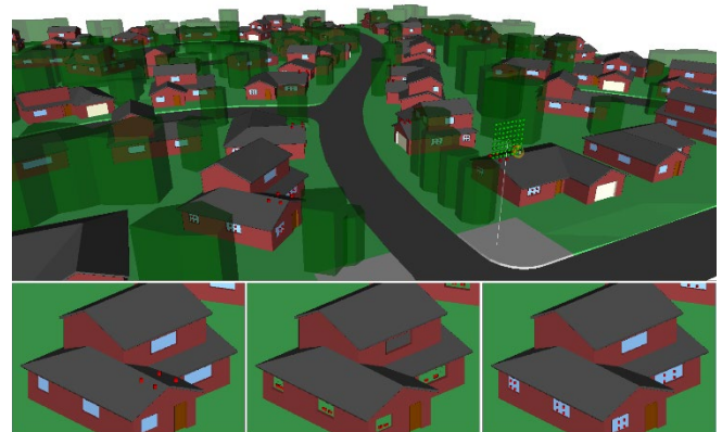
Figure 2 – Suburban FWA Scenario with 3 alternative CPEs: roof-top (left), indoor window sill (middle), and exterior window mount (right)
