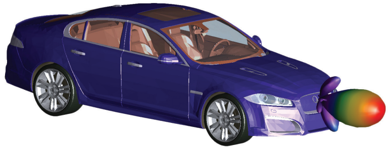
Radiation pattern for a Long Range Radar sensor.
