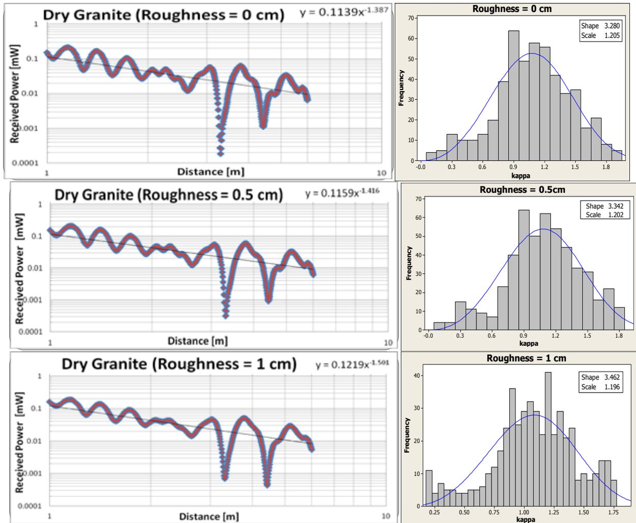
Fig. 3. Received Power vs. Distance for each surface roughness of the Dry Granite material, also displaying n-value as exponent of power law fit (right). Histogram of field amplitude deviation w.r.t. to the straight line, compared to a Weibull distribution.
