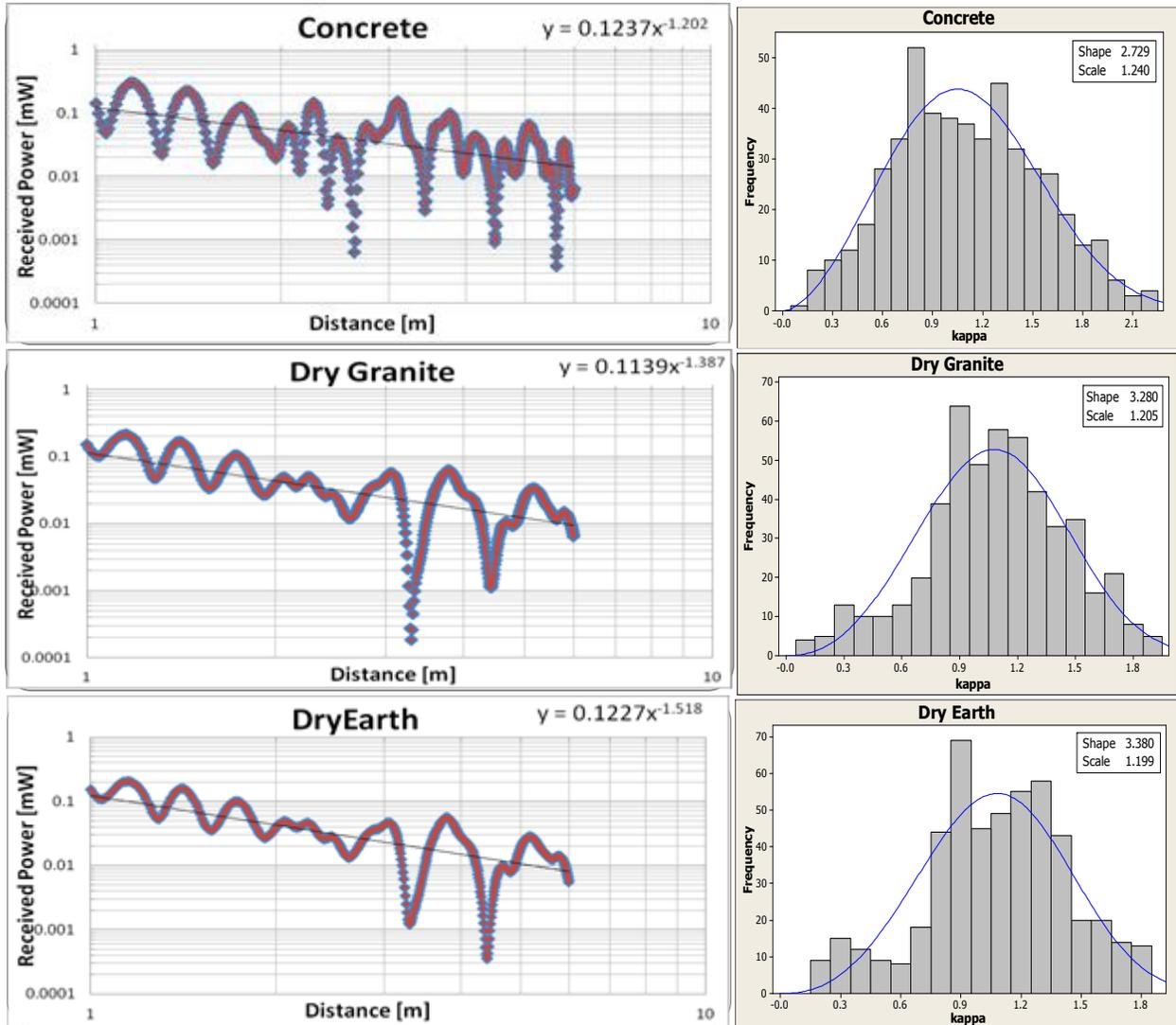
Fig. 2. Received Power vs. Distance for each material, also displaying n-value as exponent of power law fit (right). Histogram of field amplitude deviation from the straight line fit, compared to Weibull distribution.
