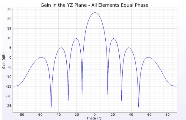
Figure 3: A line plot of the gain in a cross-sectional cut of the array pattern for the case where all patches are fed in-phase with equal amplitudes. The peak gain is just over 23 dBi and the 3 dB beamwidth is about 12 degrees.
