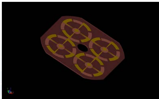
Figure 2: A detailed view of the center magnetic dipole array is shown. The four elements are printed on the top and bottom of the substrate material and are fed at the centers.
