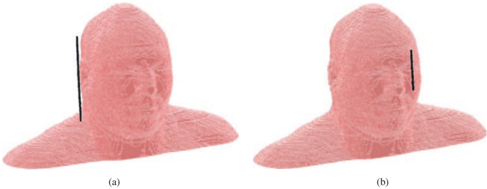
Figure 1. Example of antenna–head geometries: (a) 900 MHz dipole near the ear; (b) 1800 MHz dipole in front of the eye.
